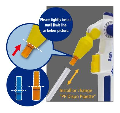
Please install or change "PP Dispo Pipette" while leaving attached dedicated adapter(with filter) attached.
